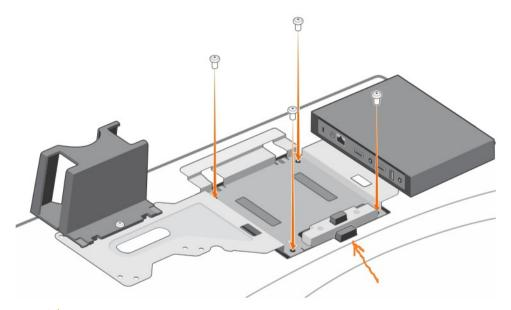
CAUTION: If you need to remove the P-series mount, remove monitor screws and then press the lower quick release button on the monitor, not the upper release button on the mount.
