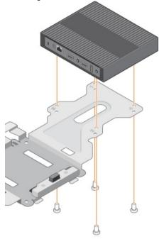
△ CAUTION: The power button should face outwards and air vents should be on top end for proper heat dissipation.
